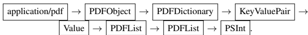
Figure 8. M\mu PDF's parse tree derivation of a byte representing an integer in a list of lists that is a value in a PDF dictionary in a PDF object.
